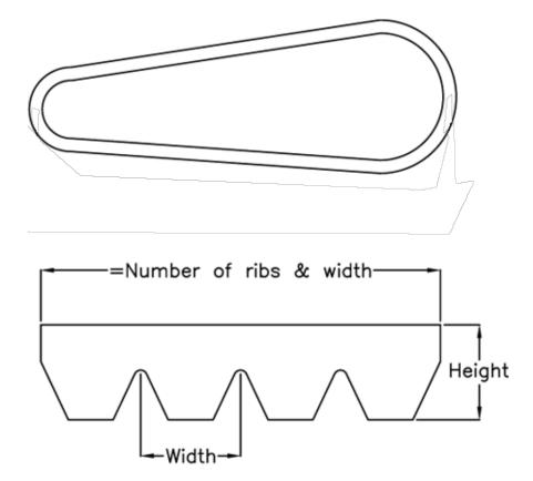
$\begin{array}{ll} \text{Datum Llength} = 2705 \\ \text{Height} &= 9.5 \\ \text{Number of ribs} = 20 \\ \text{Pitch} &= 4.7 \end{array}$
